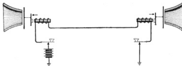
Fig. 6. Telegraph Equipment Converted into Telephone Equipment
