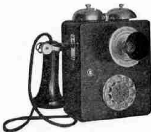
Fig. 399. Wall Set for Two-Wire System
