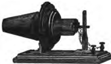
BELL'S CENTENNIAL DOUBLE POLE MEMBRANE TELEPHONE. (Same size as the single pole telephone.)
