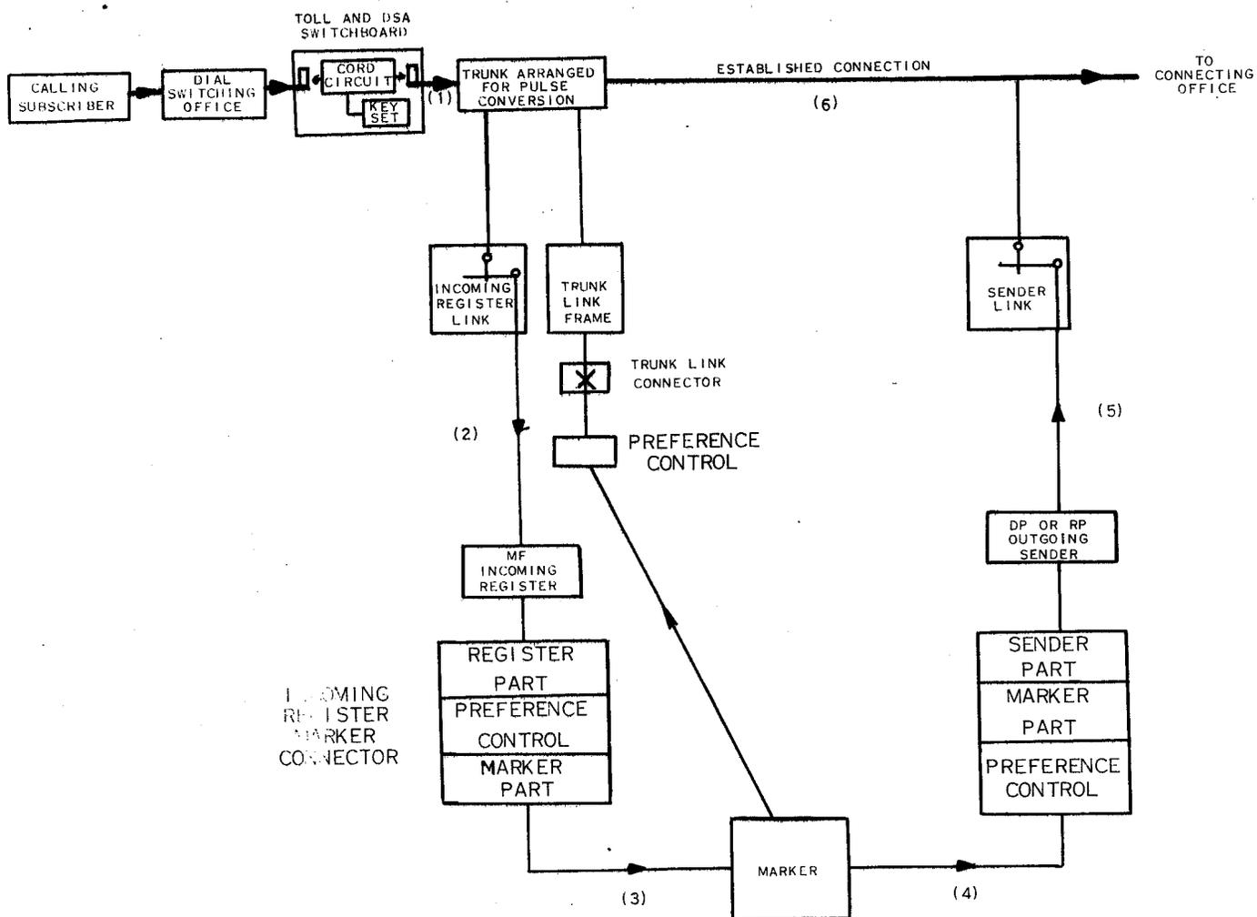
Figure 8-20 Pulse Conversion Operation
