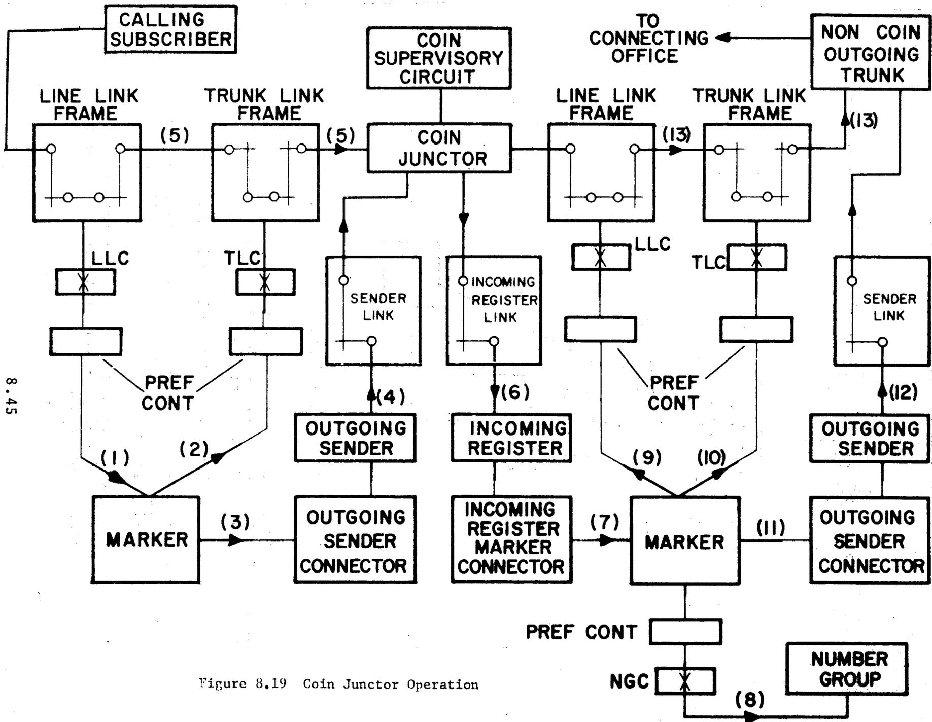
Figure 8.19 Coin Juncture Operation
