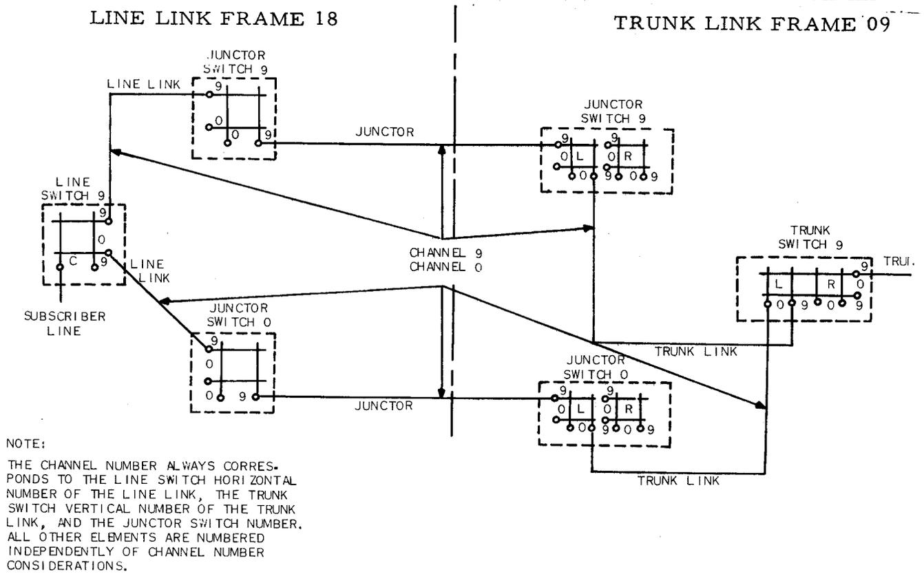
Figure 8-8 Channels for 20 Line Link-10 Trunk Link Frames
