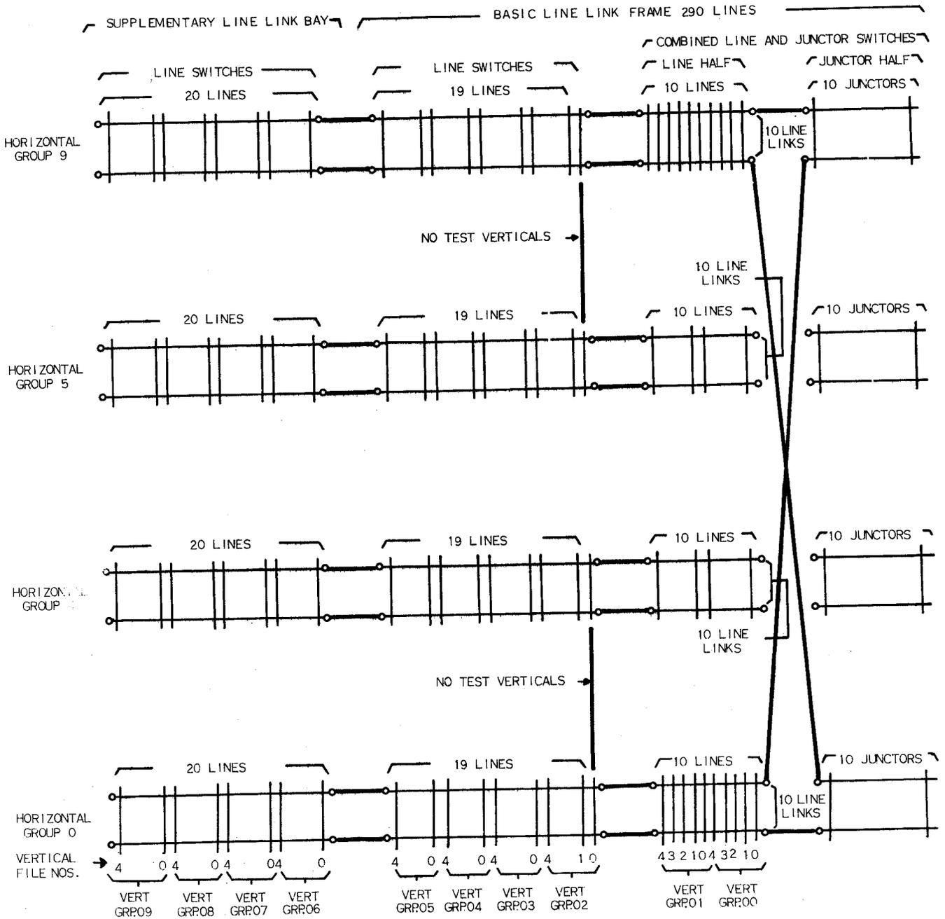
**Figure 8-3 Line Link Frames Schematic Frame Arranged for 490 Lines**
