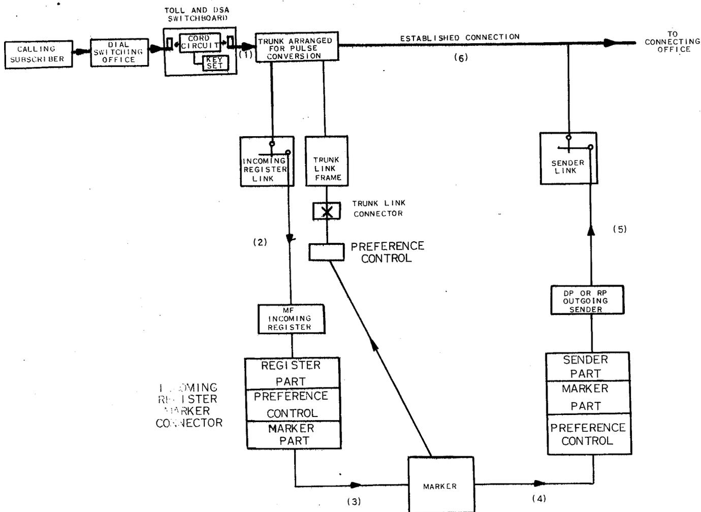
Figure 8-20 Pulse Conversion Operation
