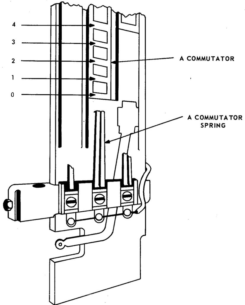
Figure 5-16 "A" Commutator Segments
