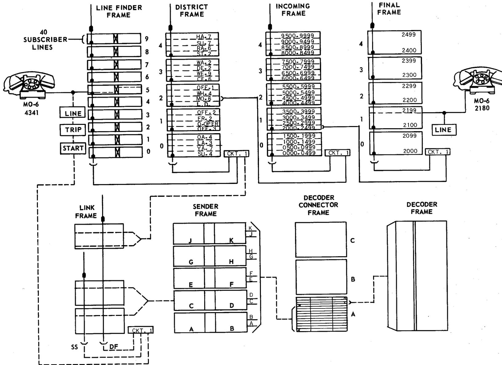
Figure 5-15 Plan of Direct Mechanical Selection
