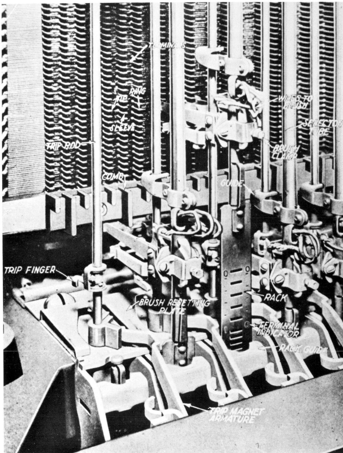
Figure 5-4 Panel Type Selecting Mechanism
