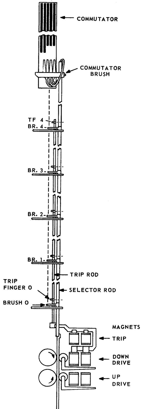
Figure 5-3 Selector Rod, Drive Mechanism, and Clutch Assembly
