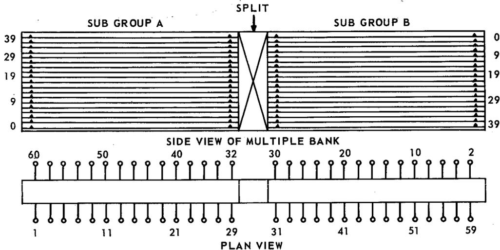
ARRANGEMENT OF MULTIPLE BANK USED FOR TERMINATING 400 LINES PER FRAME
