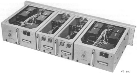
FIG. 5-20. Power supplies and paralleling units.
